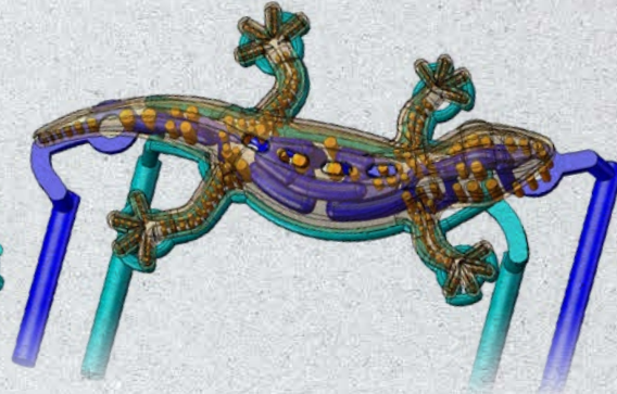
Contour-following temperature control on the injector side. Controllable in two different cycles.
