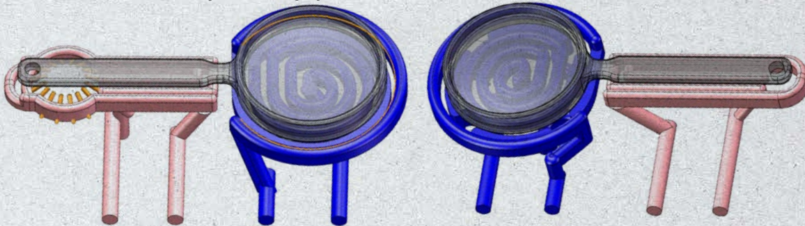
The variothermal, conformal tempering channels are located on the cavity half, divided into two zones.
